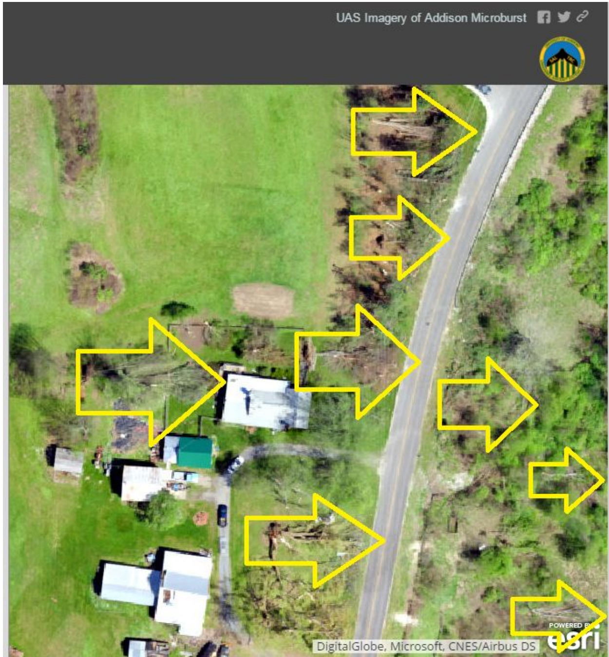
Figure 17: University of Vermont UAS Team imagery around the intersection of Potash Bay Rd and Lake St. The yellow arrows show where trees have been blown down by the microburst all in a straight line from west to east.
